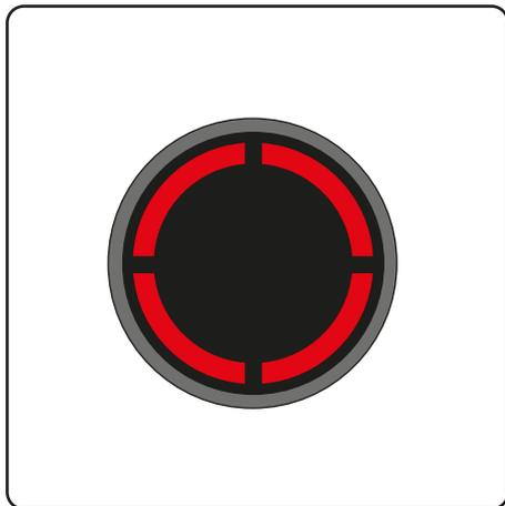
If the brush bar jams during use, the product will stop and the LEDs will appear red. You will need to remove and clean the brush bar.
