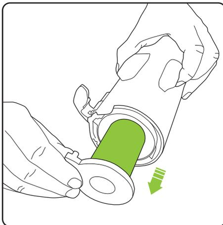
Pull the filter out of the filter housing. Tap the dirt from the filter and tip any dirt from the filter housing. Wash the filter if necessary.
