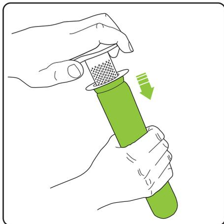
Remove the filter from the inner shroud, by twisting and pulling. Tap the inner shroud over a bin to remove any excess dirt.
