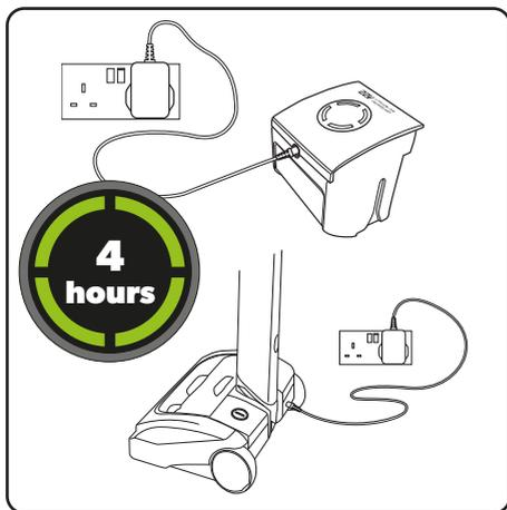
The battery can be charged whilst it's in the product, or when it's off the product. The battery can be charged from flat in 4 hours. The state of charge indicator will show 4 solid green lights when it is charged.
