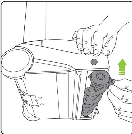
Re-insert the brush bar, starting by the end furthest away from the button. Then line up and push the brush bar into the product until it clicks into place.
