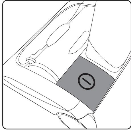
The power button is located on the left hand side of the head assembly.
