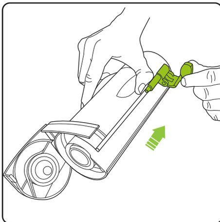
Pull the green lever back towards the bottom of the bin. Close the bin lid and reinsert the bin into the product.
