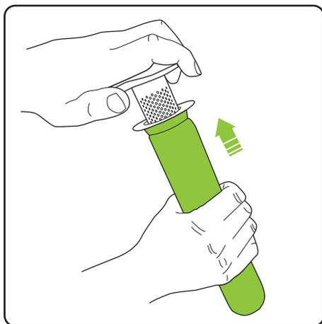
Slide the filter onto the inner shroud.
