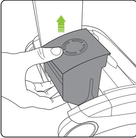
Before checking for a blockage, remove the battery.
