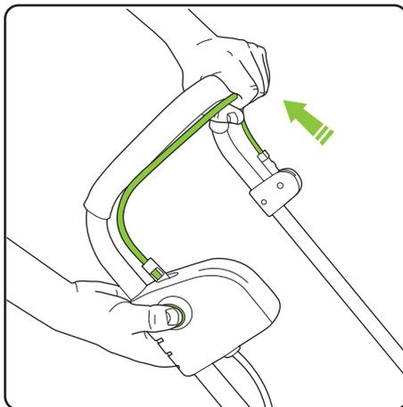
Pull the lever to the handle to start the mower. Releasing the lever will stop the mower.
