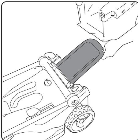
Whilst still lifting the protective flap, lift and pull the grass box towards you to remove from the mower.
