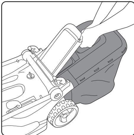
Lift the protective flap at the rear of the mower and grasp the green handle attached to the grass box.
