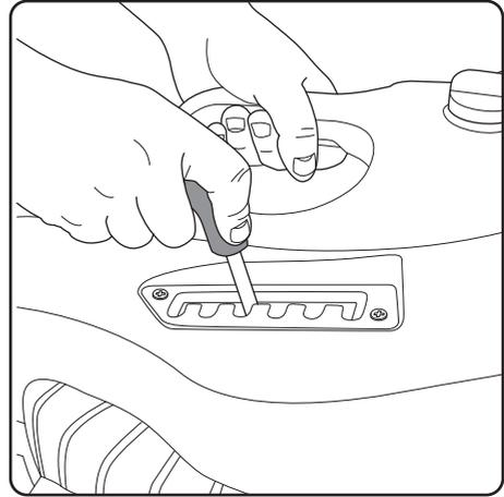
To adjust the height, hold the lever firmly and move it into the notch required.
