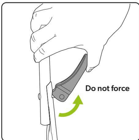
Push the locking handle 90 degrees towards the pole. If the locking handle struggles to lock then lower the locking handle, twist backwards to loosen and try again.
