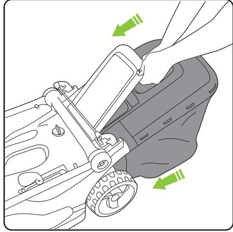
Insert the grass box into the back of the mower.
