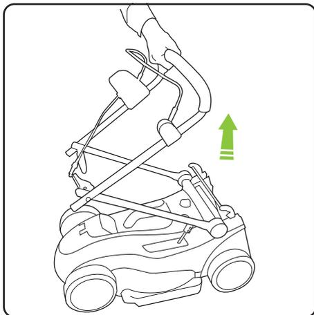
Put the grass box to one side and take hold of the mower's upper handle. Pull upwards to extend the handle assembly.
