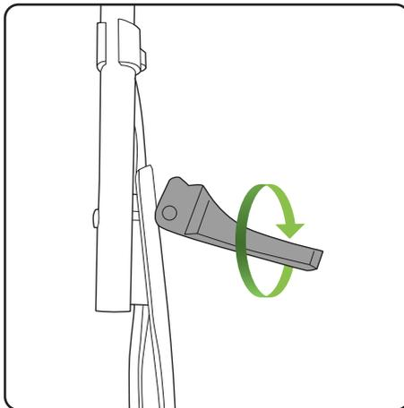
Twist the locking handles to tighten
