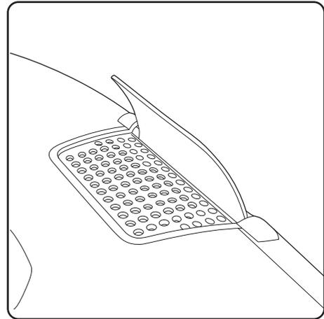
When the filling indicator flap closes, it is time to empty the bin. Note: if the bin over-fills, the grass chute will clog and the flap will close again.
