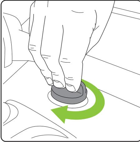
The mower will not work without the safety key. Rotate it 90° clockwise to operate.
