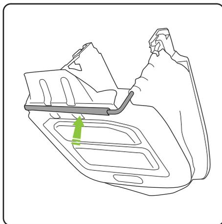
Then push the metal rod into the clip underneath the grass bin.
