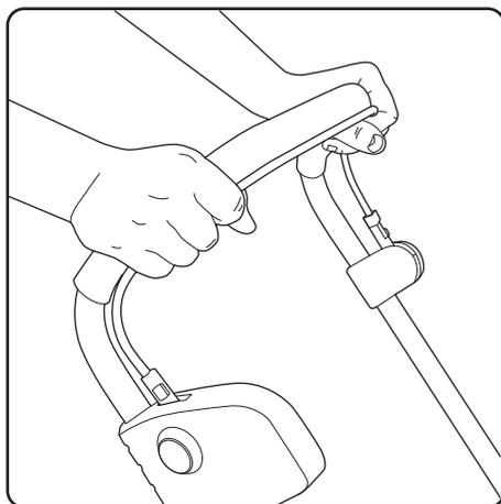
Once the mower is activated, you can release the safety button.
