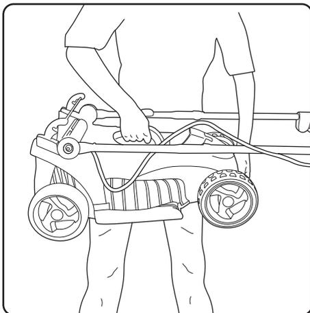
Before carrying the mower, make sure the safety key is removed to avoid starting it accidentally. The easiest way to carry the mower is by holding the middle carry-handle and the front of the mower.
