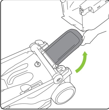
To fit the grass box onto the mower, lift up the protective flap.
