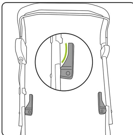
When correctly assembled the locking handles will be located on the inside of the handle frame with the curved section of the locking handle on the inside.
