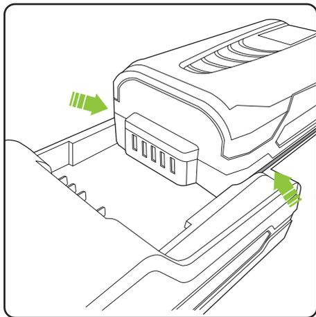
With the 'G' logo facing upwards on the battery, line up the runners on the sides of the battery with the runners on the battery charge stand and slide onto charger.
