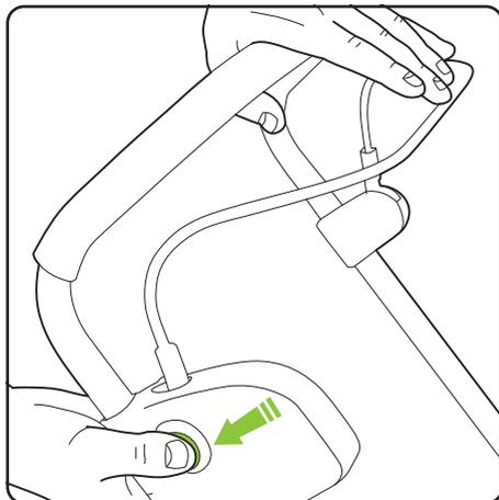
To operate the mower, press and hold the green safety button and then pull the lever under the handle.
