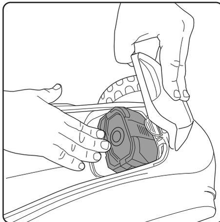
Ensure the battery is firmly pushed down and clicked into place in the battery housing.
