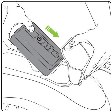
Ensure the 'G' logo is facing upwards when you slide the battery into the battery housing. It will push firmly into place once fitted correctly.
