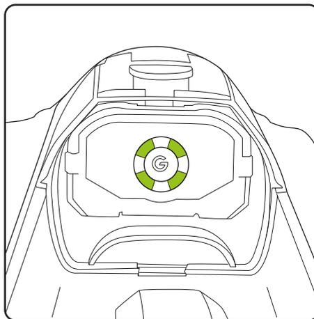
The state of charge indicator on the battery will be visible through the visor.
