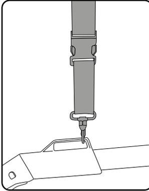
Attach the clip to the loop on the of the handle and clip the harness to this.
