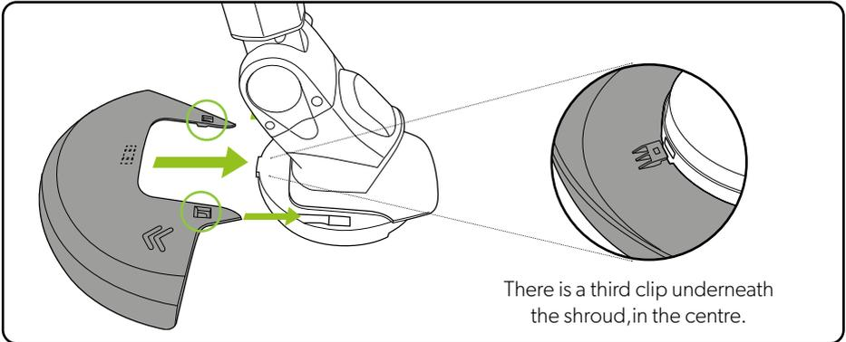
**Attach the shroud first.** Align both clips on the shroud to the holes on the trimmer head and simultaneously push them into place.
