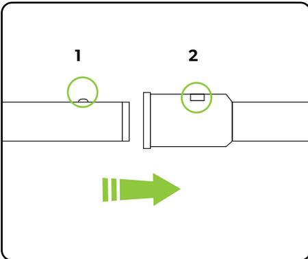
Assemble the two parts of the handle. When the pole is fully inserted, the button (1) will pop up into the aperture (2).
