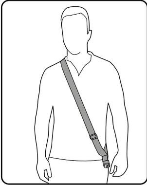
The harness can be used to bear the load of the product. The sling passes over your head and rests on your shoulder - use the sliding adjuster to ensure the harness fits you comfortably.
