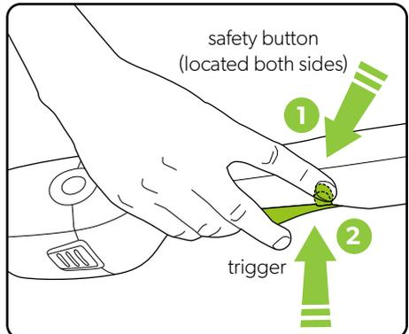
Push and hold the safety button on either side, then press the trigger to operate. When you release the trigger the trimmer will stop.
