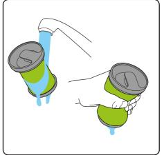
Wash the filter under a tap, squeeze it out then let it **dry completely** before using it. Recommended water temp 40°C do not use any detergent. (You can buy more at **www.gtech.co.uk**)
