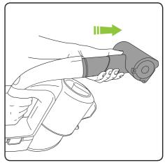
Gently pull the Power Brush from the Multi to remove. The battery should be removed when changing attachments.
