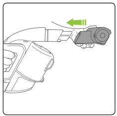
Make sure the terminals on the Power Brush and Active nozzle are correctly lined up and gently push the Power brush onto the Active nozzle. The battery should be removed when changing attachments.
