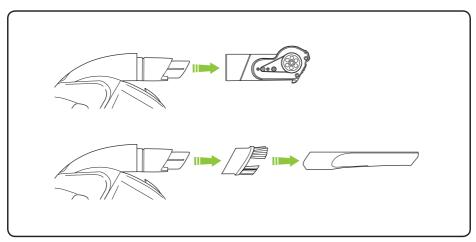
An active nozzle is built into your Multi. The dusting brush, crevice tool, and power brush all attach to the active nozzle.
