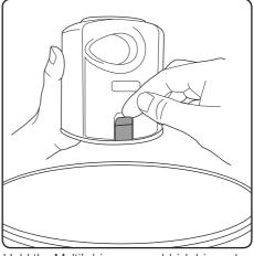
Hold the Multi's bin over a rubbish bin and release the latch to empty the dirt. A gentle tap will help. Remove the filter and tap off the excess debris each time you empty the bin.
