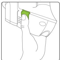
Press the green buttons and pull to remove the battery. The battery can be charged on or off the main unit. If you want to buy a spare battery go to www.gtech.co.uk or call 01905 345891
