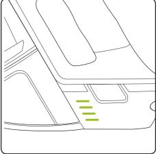
The battery state of charge indicator shows how much charge the Multi has. As you use the product, the green lights will turn off in a downwards direction.
