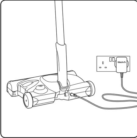
Plug in the charger and connect the jack to the socket at the rear of the sweeper. A full recharge will take 16 hours. Do not charge for longer than 24 hours.
