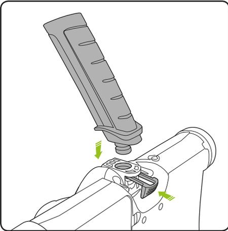
Place the lower handle into the socket.
