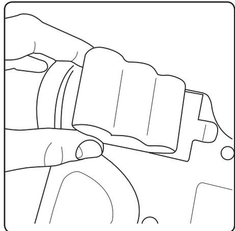
Put the battery back into the compartment and replace the cover.
