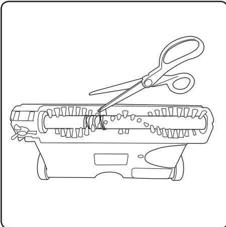
From time to time you may need to remove hair and thread from the brush bar. Take off visor and use a pair of scissors to remove the hair.
