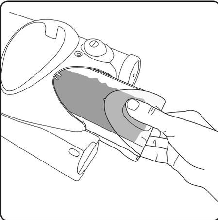
Remove the dust tray by pinching the window slightly, and pulling out.
