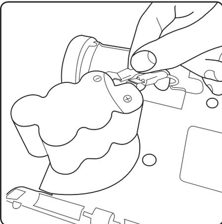
Lift out the battery pack. Straighten up the cable connectors so you can handle them more easily.
