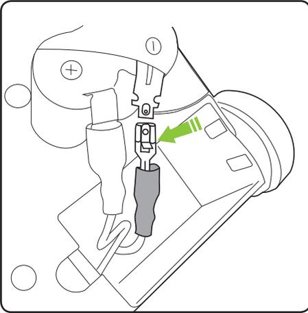
Gently press down fixing latch on cable connector.
