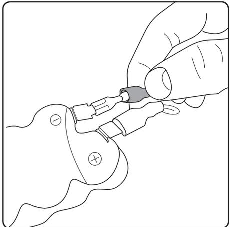
Slide plastic cover off the **BLACK** cable connector **ONLY**. Leave cover on the red cable connector.
