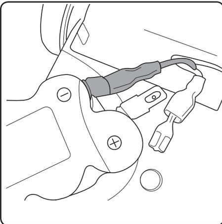
Re-attach the wires to the new battery, attaching the BLACK wire first. Fold the terminals back along the battery.
