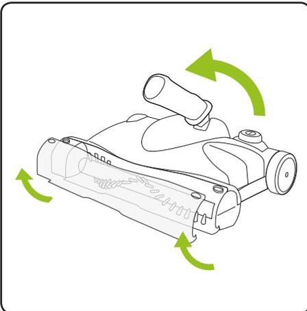
Remove the visor by unclipping the bottom outer edges at the same time then lifting off. Push lower handle fully forward.
