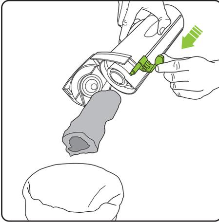
Hold the AirRAM K9's bin over a rubbish bin and push the green lever towards the lid to empty the dirt.
