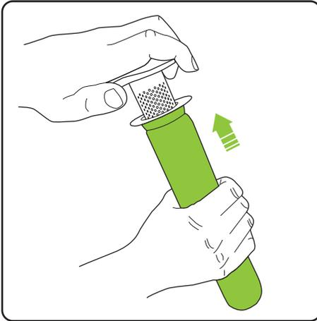
Slide the filter onto the inner shroud.
