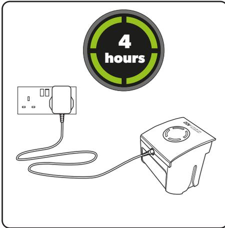
Plug the charger into the mains and connect it to the battery. Switch on at the mains. The battery can be charged from flat in 4 hours. The state of charge indicator will show 4 solid green lights when it is charged.
