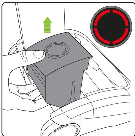
If the brush bar jams during use, the AirRAM K9 will stop and the LEDs will appear red. Before checking for a blockage, remove the battery.
