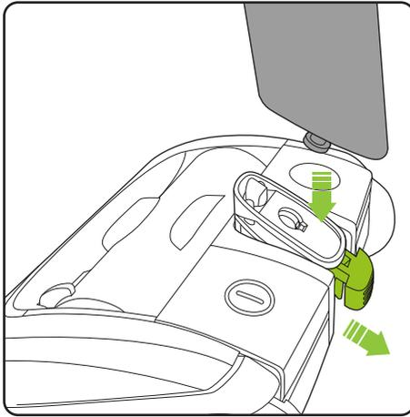
To attach the lower handle to the head assembly, insert the metal pin on the lower handle into the hole located on the pivot yoke. Make sure the green locking clip is pulled out to allow the lower handle to fit.
