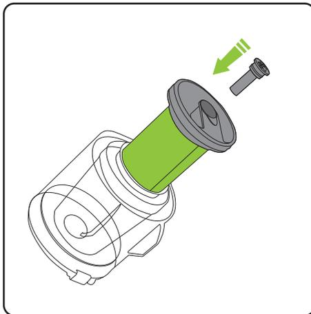
Ensure tab is refitted on to filter before using.
