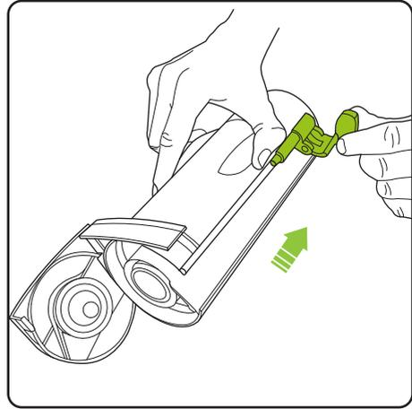
Pull the green lever back towards the bottom of the bin. Close the bin lid and reinsert the bin into the AirRAM K9.
