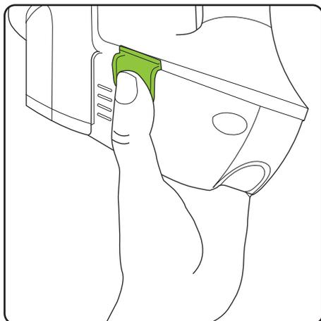
Press the green buttons and pull to remove the battery. The battery can be charged on or off the main unit. If you want to buy a spare battery go to [www.gtech.co.uk](http://www.gtech.co.uk) or call **01905 345891**
