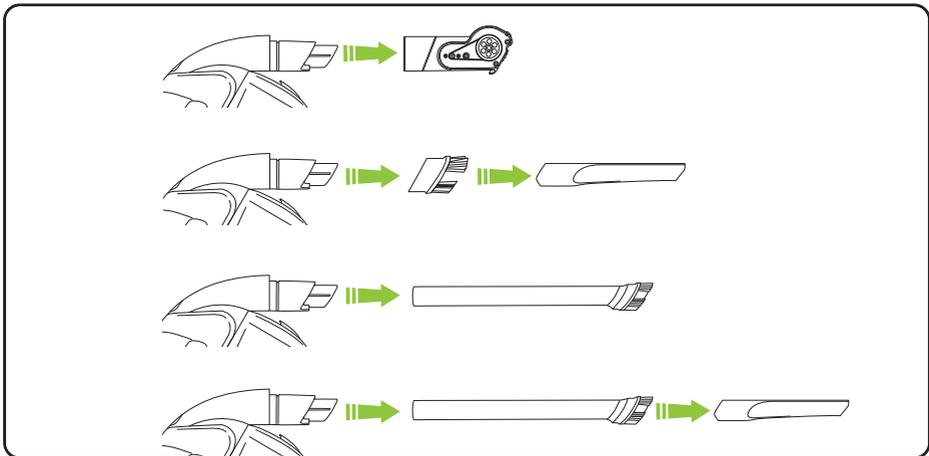
An active nozzle is built into your Multi K9. The power brush, dusting brush, crevice tool and extension tube all attach to the active nozzle.
