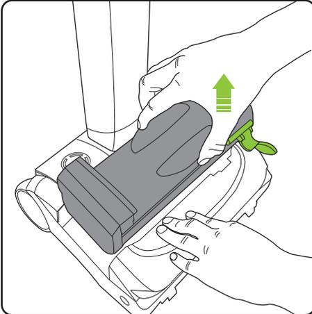
Holding onto the AirRAM K9 with one hand, pull the bin handle and lift the bin out of the AirRAM K9.
