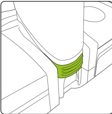
The green locking clip, when correctly fitted, will click and hold the lower handle in place. Should the handle assembly need to be removed the clip can be pulled out to unlock the lower handle. The green locking clip remains permanently attached to the head assembly.
