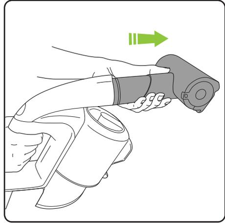
Gently pull the Power Brush from the Multi K9 to remove. The battery should be removed when changing attachments.
