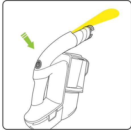
Press the button above the handle to turn the Multi K9 on and off.
