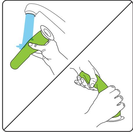
Wash the filter under a tap. Squeeze out any excess water then let it **dry completely** before reinserting into the AirRAM K9. Recommended water temperature 40°C. Do not use detergent or soaps. **Never put the bin back without filter inside. You could damage the motor.**
