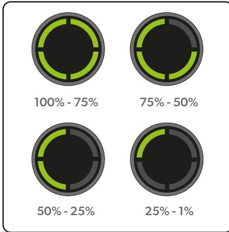
The battery state of charge indicator shows how much charge the AirRAM K9 has. As you use the product, the green lights will turn off in a downwards direction.
