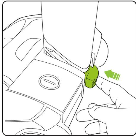
Ensure the lower handle is sitting completely flush against the yoke. Then push the green locking clip into the back of the head.
