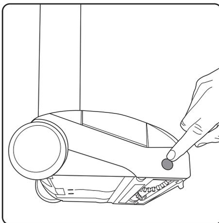
Rest the AirRAM K9 on its side and locate the brush bar button on the right hand side. Press the button inwards and then pull the brush bar out from the bottom of the AirRAM K9.
