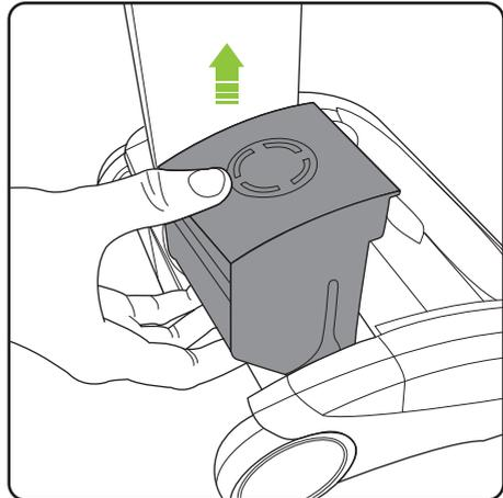
The battery can be charged whilst it's in the AirRAM K9, or when it's off the product. To remove the battery, squeeze the latch underneath and pull upwards.
