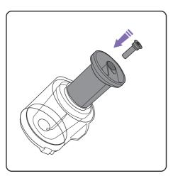
Place the new scented cartridge into the top of the filter.
