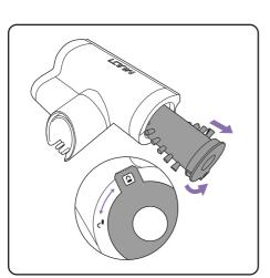
To clean the brush bar, first remove the power brush. Rotate the latch from the lock to the unlock position and pull out the brush bar.
