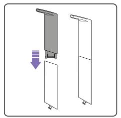
Push the two parts of the lower handle together in the orientation shown above. They will only fit one way. They will click into place and remain permanently fixed.
