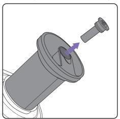
Remove the old scented cartridge by pulling it out from the housing at the top of the filter.
