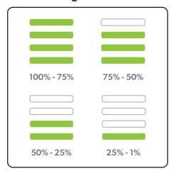
The battery state of charge indicator shows how much charge the product has. As you use the product, the green lights will turn off in a downwards direction.
