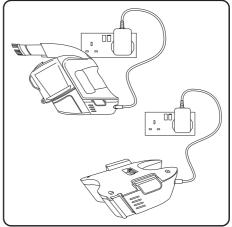
The battery can be charged on or off the main unit
