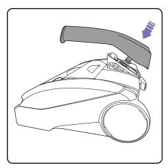
To attach the speed clean handle, insert the pin into the yoke (hole) on the AirRAM head.
