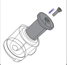
Ensure a cartridge is fitted onto the filter before using.
