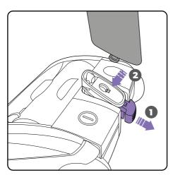
Pull out the purple locking clip to allow the lower handle to fit (the clip remains attached to the head) Insert the metal pin on the lower handle into the hole in the pivot yoke.
