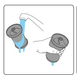
Wash the filter under a tap, squeeze it out then let it **dry completely** before using it. Recommended water temperature 40°C. Do not use any detergent or soaps. Use your spare filter while it dries. (You can get more at www.gtech.co.uk) Never operate the product without the filter inside the bin. You could damage the motor.
