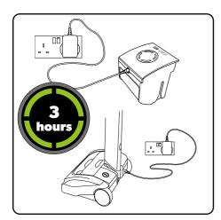
The battery can be charged whilst it's in the product, or when it's off the product. The battery can be charged from flat in 3 hours. The state of charge indicator will show 4 solid green lights when it is charged.
