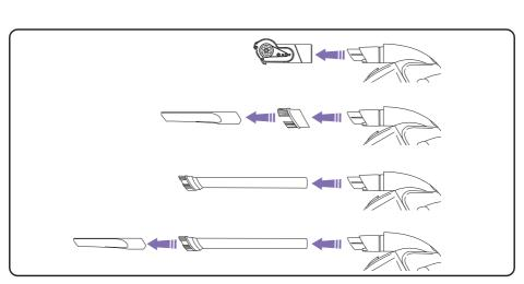
An active nozzle is built into your product. The dusting brush, crevice tool, extension tube and power brush all attach to the active nozzle.
