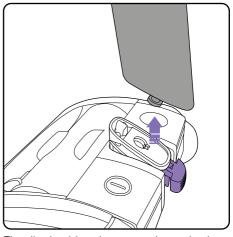
The clip should not be removed completely as it remains part of the lower body assembly.
