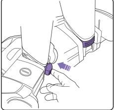
Ensure the lower handle is sitting completely flush against the pivot yoke. Firmly push the purple locking clip until it clicks fully into place. The clip can be pulled out to unlock the lower handle should it need to be removed.
