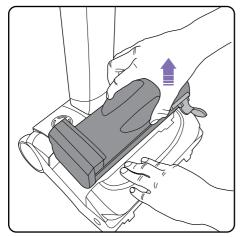
Holding onto the product with one hand, pull the bin handle and lift the bin out of the product.
