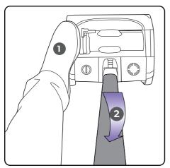
Without pressing the power button, place your foot on the left side of the head (1) and pull the handle back (2).
