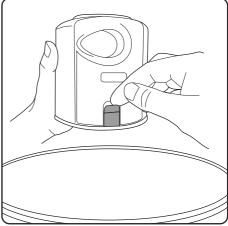
Hold the bin over a rubbish bin and release the latch to empty the dirt. A gentle tap will help. Remove the filter and tap off the excess debris each time you empty the bin.
