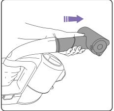
Gently pull the Power Brush from the product to remove. The battery should be removed when changing attachments.
